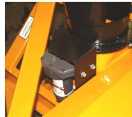
**Step 9 - Install shield.** With the remaining two 3/8" bolts and nuts, install the shield over the motor assembly. Make sure the shield does not interfere with any moving parts, like the gear or the spout.
