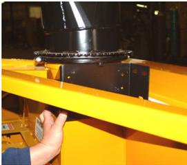
**Step 2 - Position Bracket.** Hold the mounting bracket 1/4" under the spout ring and against the main housing.
