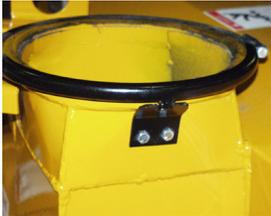
**Step 1 - Remove Retainer.** If your fan output has a ring retainer bracket, remove the bolts and the bracket.
