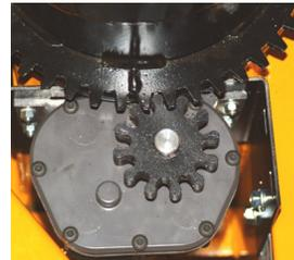
**Step 8 - Gear Alignment and Mesh.** Position the motor assembly so the gears have about 1/4" gap between the teeth. This gap will allow for small discrepancies as the spout turns. After setting, tighten all four bolts. Adjust the position of the gear on the shaft so it is centered on the spout gear. Tighten the set screws.
