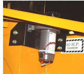
**Step 7 - Attach Bracket to Housing.** Hold the mounting bracket in position and insert four 3/8" bolts into the holes and start the nuts. Leave the nuts loose for gear alignment.
