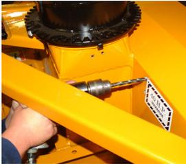
**Step 4 - Drill Holes.** Using a 13/32" bit and drill, drill the 2 holes in the main housing and the two in the fan housing. After drilling, the holes may need filing to remove any sharp burrs.
