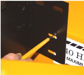
**Step 3 - Mark slots.** Use a pencil to trace the slots onto the main housing and fan housing. Center punch the slot position toward the right end of the slot.
